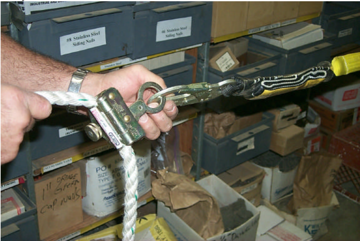
Picture of how lanyard is assembled to safety vest.
