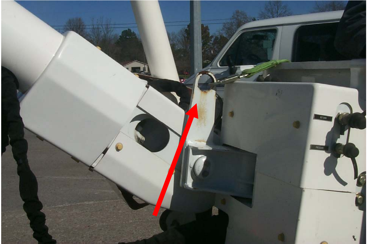
Photograph depicts the attachment of the boom to the bucket and the eye hook for harness attachment
