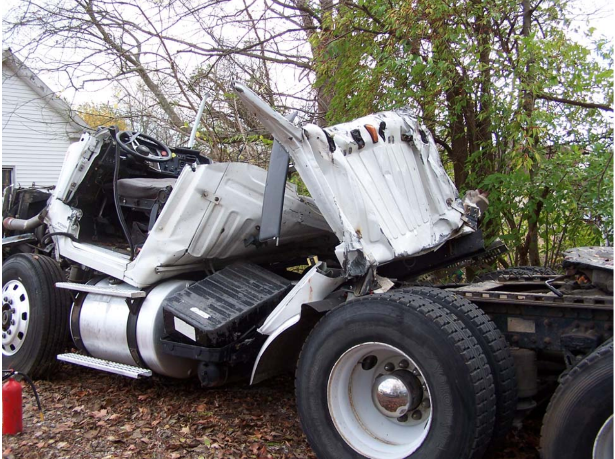
Cab of semi-tractor at towing company after collision. Top of cab was cut away with torches. Seat belts were cut to free both occupants.
