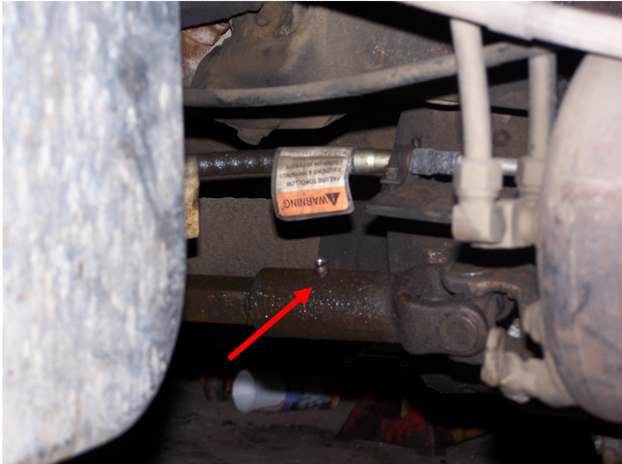
Photograph of grease fitting on universal joint power-take-off drive shaft that caught worker's coat
