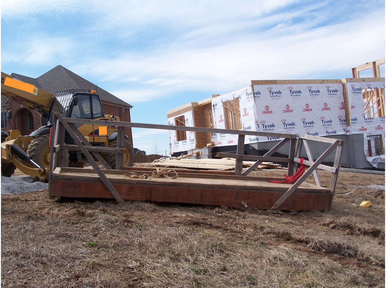
Picture of side used to lift homemade platform. Notice there are no cleats for forks on this side.
