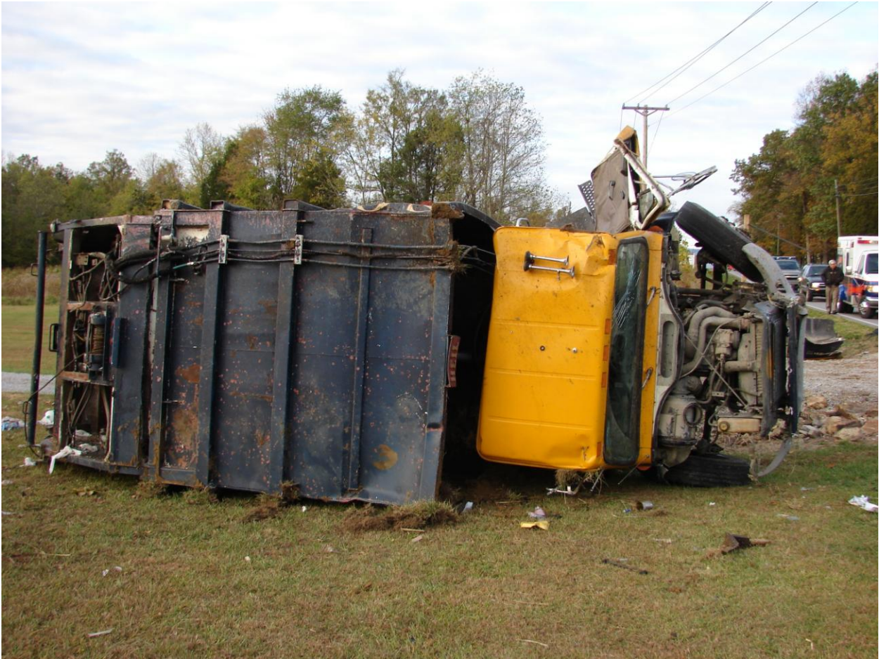
Photograph of solid waste truck where and how it came to rest after rolling end-over-end. Photograph courtesy of law enforcement.
