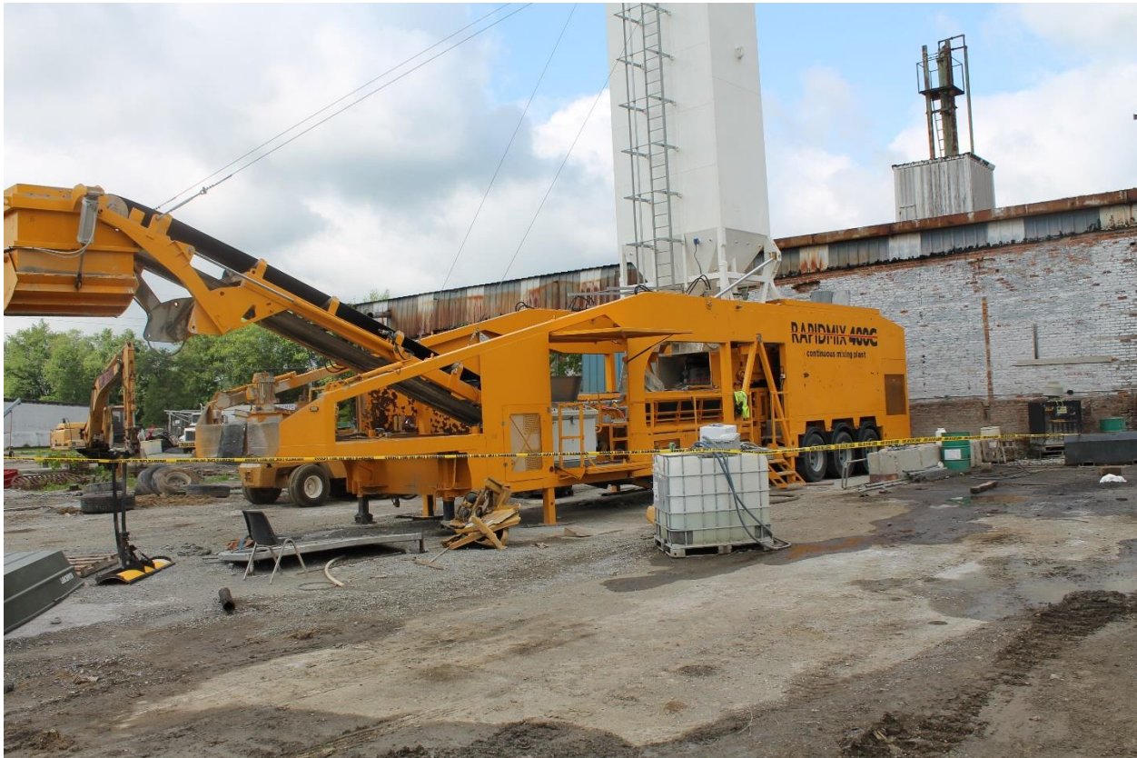
Photo #1 Rapidmix 400 C Continuous Mixing Plant. OSHA
