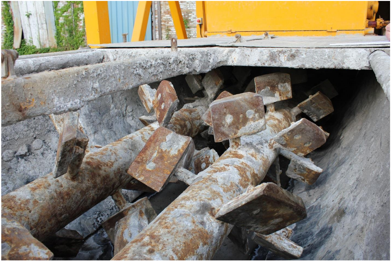
Photo 4: the auger mixer paddles victim fell into.
