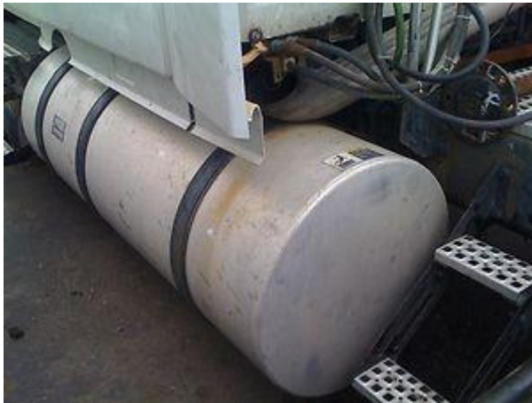
Figure 7. Stock photo of a side mounted fuel tank commonly found in semi-truck designs.
