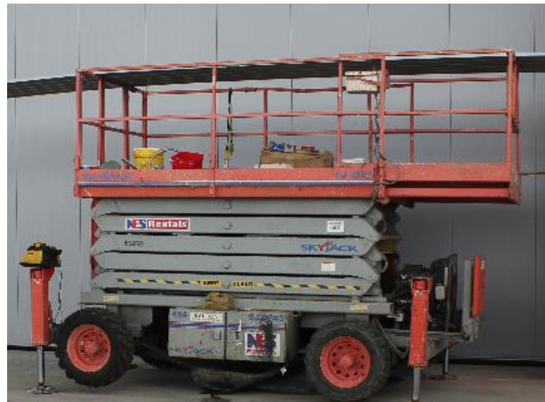
Figure 4. Skyjack SJ8243 Scissor lift which was located on the construction work site that would have been appropriate for lifting the personnel. This lift had a maximum height of 43 feet.
