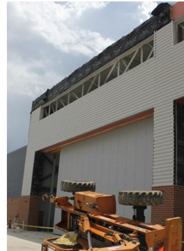
Figure 1. Telescopic forklift overturned at jobsite.
