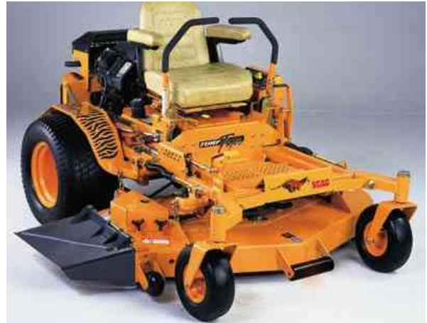
Figure 3. Stock photo of a Scag brand Turf Tiger zero-turn riding lawn mower without ROPS installed.
