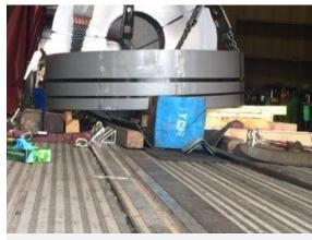
**Figure 8.** Steel coil that fell on and crushed truck driver, on flatbed trailer.
