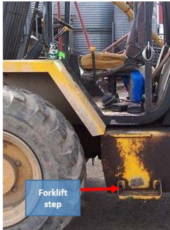
Figure 4. The victim was riding on the forklift's side step at the time of the incident.
