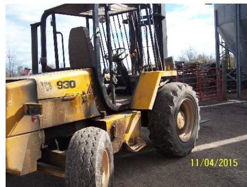
Figure 1. Rough Terrain JCB 930 forklift.
