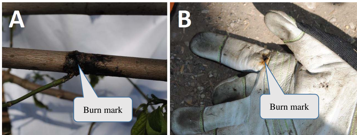
Figure 7. One of three burn marks on the branch (A); burn mark on the victim's glove (B).
