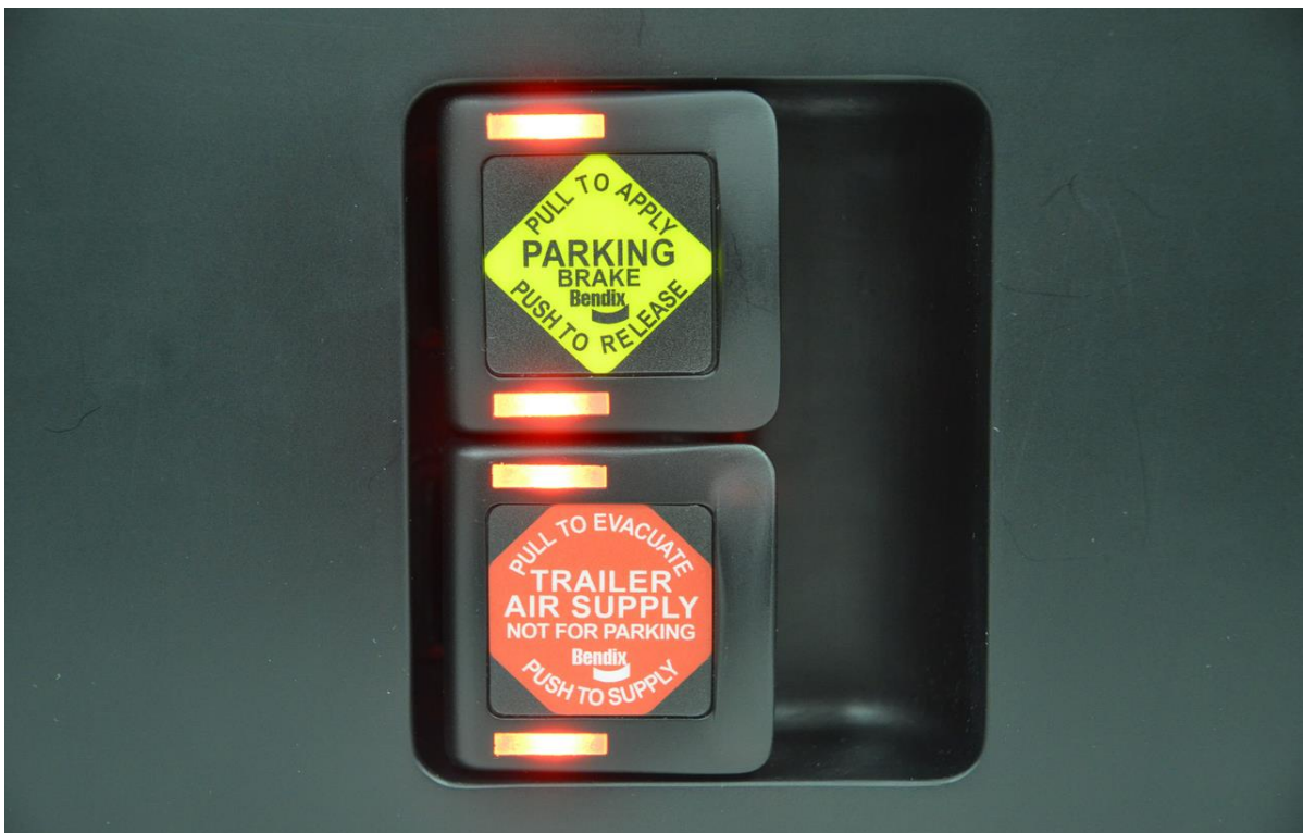
Picture 2. Picture of Bendix Intellipark LED brake interface. Retrieved from https://www.oemoffhighway.com/drivetrains/brake-system/press-release/21060126/bendix-commercial-vehicle-systems-llc-bendix-pilot-testing-intellipark-electronic-parking-brake-with-fleets
