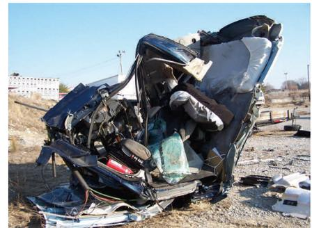
**Case 3:** A 46-year-old male driving a sealing and striping truck for an asphalt company died after the rear passenger tire failed. The truck overturned three to four times and the driver, who was not wearing a safety belt, was thrown from the vehicle and died at the scene.
