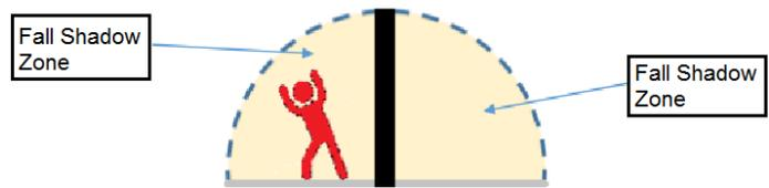
Employees should stand clear of the area surrounding cargo in which it is reasonably foreseeable that a tip over would result in crushing/struck-by injuries. Workers are especially vulnerable to this zone when the cargo is being moved.
