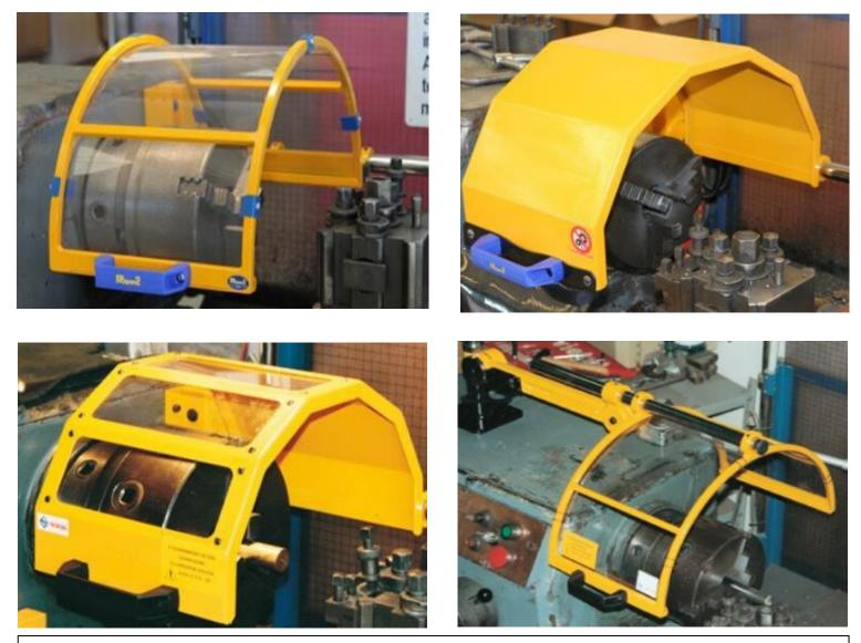
Photo 6, 7, 8 & 9. Examples of aftermarket guarding systems on similar machines.<sup>4</sup> Photos obtained from <u>https://www.eputec.de/en/safety-guards/safety-guards/safety-guards-for-lathes/</u>
