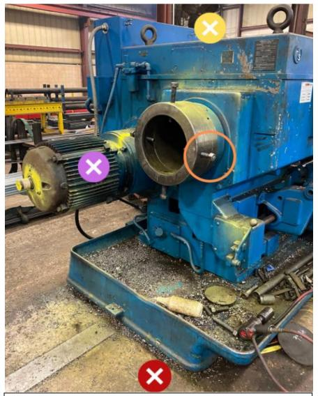
Photo 5. The **red X** indicates the position of the victim when he attempted to reach on top of the machine. The **yellow X** indicates the location believed to be where the glove was located. The **purple X** represents the lathe motor which the victim struck multiple times after becoming entangled. The **orange circle** is highlighting the chuck which caught the victim's clothing. Photo is property of KY FACE.
