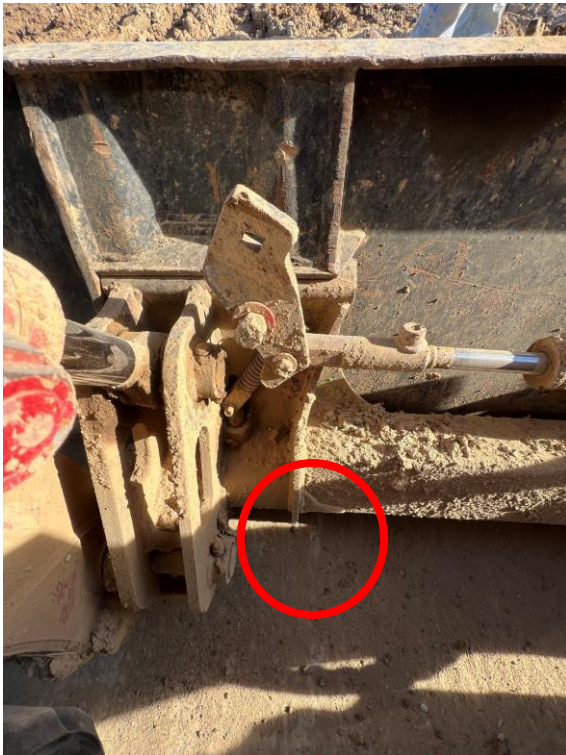
Photo 7. Skid-steer locking pin (Courtesy of KY FACE).
