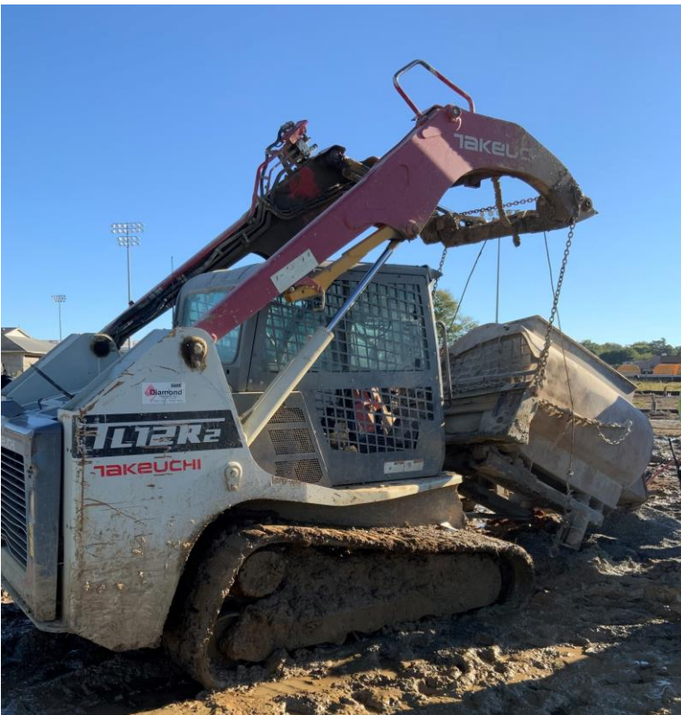
Photo 5. Skid-steer with twin-fork attachment and bucket (Courtesy of coroner).
