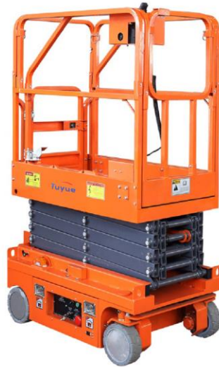
Photo 4. Stock photo depicting the type of scissor lifts that were available for use at the job site.
