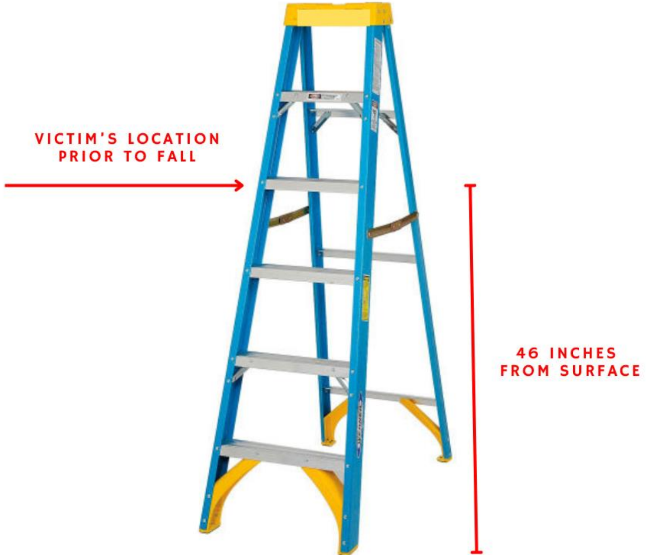
Diagram 1. Diagram depicting the type of ladder utilized by the victim, the step he was standing on, and the distance the victim was from the surface. Diagram created by and property of Kentucky FACE.
