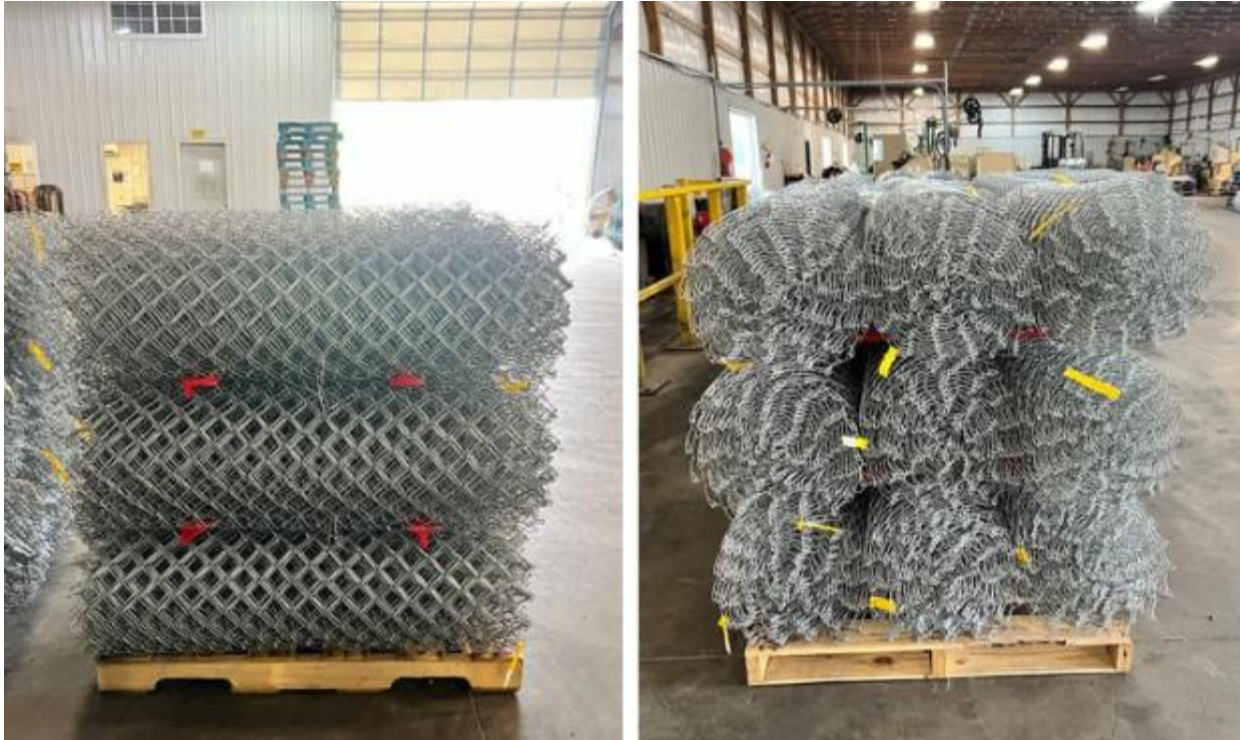
Photos 2 and 3. Photos of finished panels measuring 50 feet long by 4 feet wide. Photo property of Kentucky FACE.
