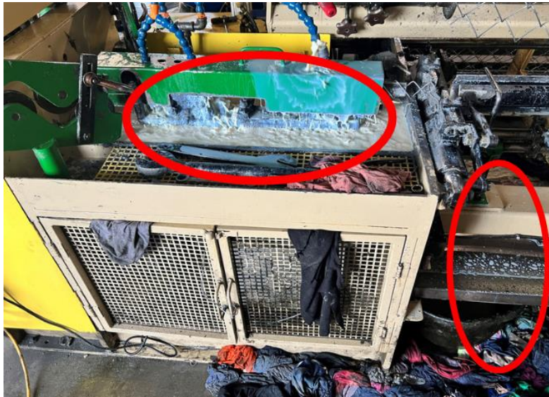
Photo 5. Photo showing lubricant used in the manufacturing process and towels utilized for cleaning. Photo property of Kentucky FACE.
