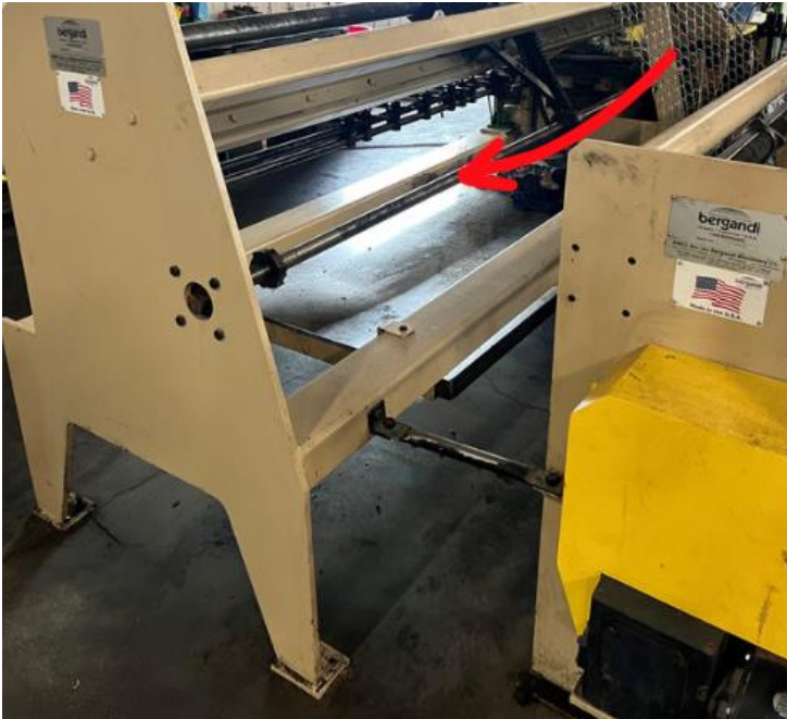
Photo 7. Red arrow indicating the horizontal shaft in which the victim's hair was entangled. Photo property of Kentucky FACE.
