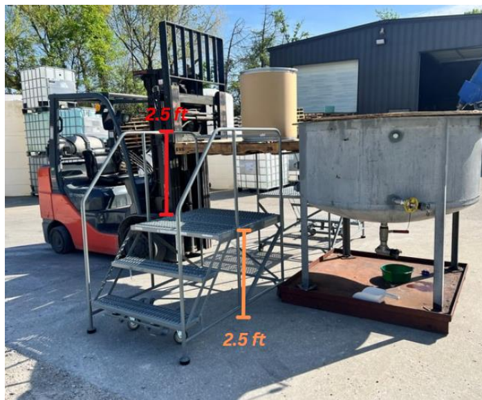
Photo 5. Photo showing new ladders and process implemented by involved company. Photo property of Kentucky FACE.
