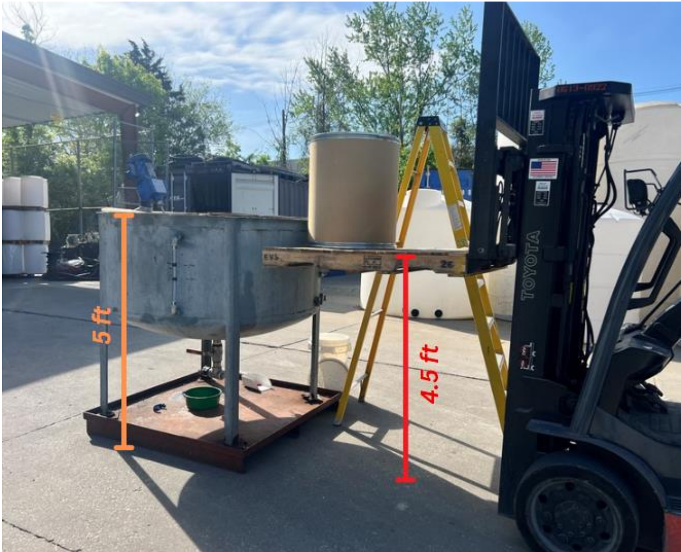
Photo 2. Photo of commercial grade mixer, 132-pound product drum, ladder, forklift, and pallet, which were utilized when the incident occurred. Scene was reconstructed for investigation purposes. Orange line represents height of commercial grade mixer from the surface below. Red line represents height of the elevated platform the victim was standing on to the surface below. Photo property of Kentucky FACE.
