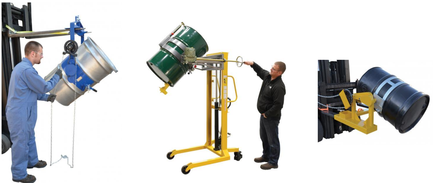
Photo 4. Photos showing various drum handling device options. Images obtained via Google search.
