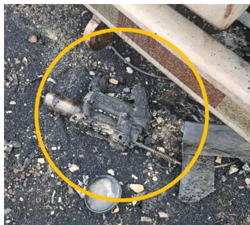
Photo 5. The electric grease gun used in the incident.
