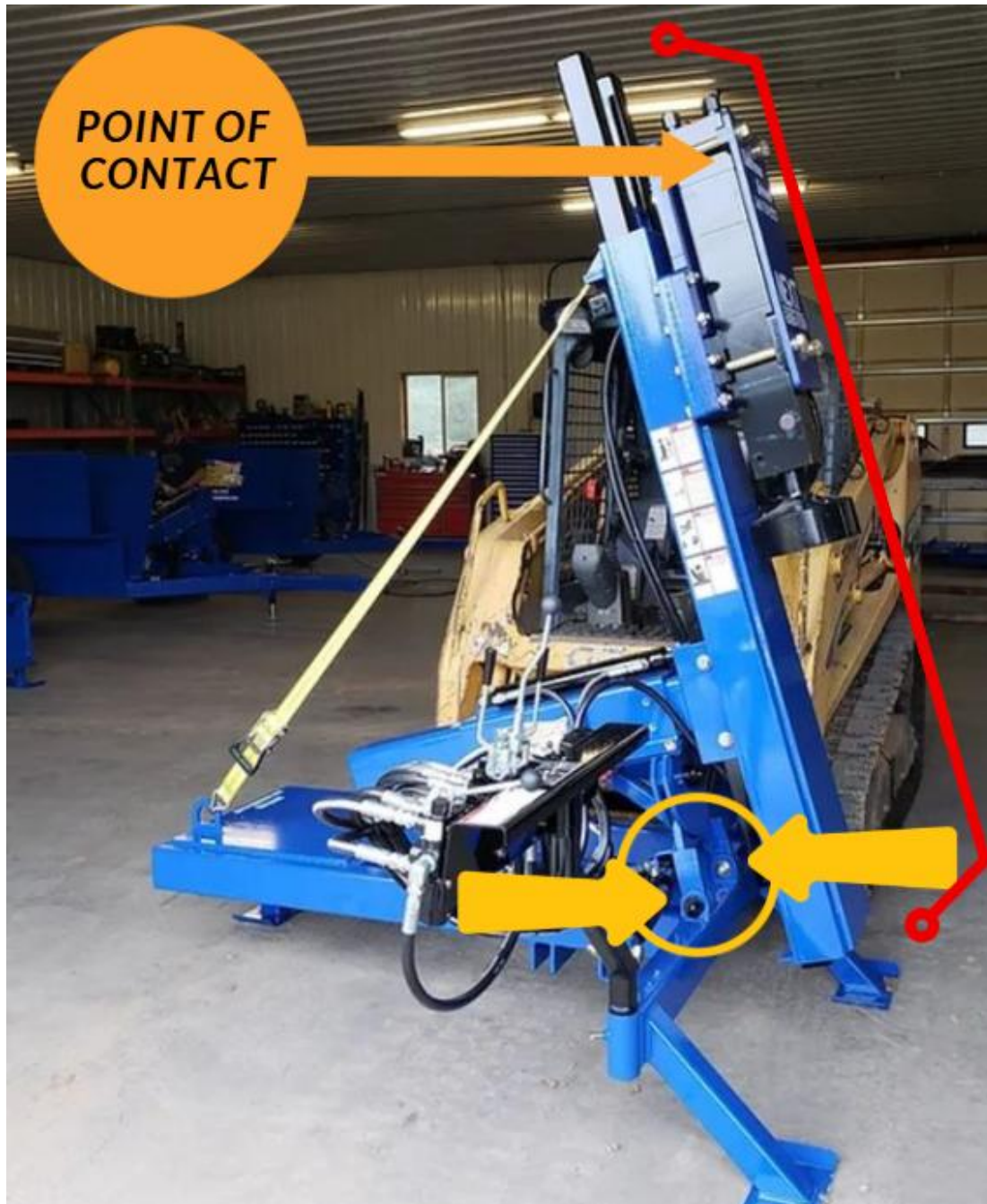
Photo 8. Photo showing a similar post-driver. Yellow arrows depict points where machine broke from base. Red lines show the driver arm and head which fell towards the victim. Orange arrow indicates the point of contact with the victim's back/shoulder area. Photo obtained via Google search, modified to aid in investigation.
