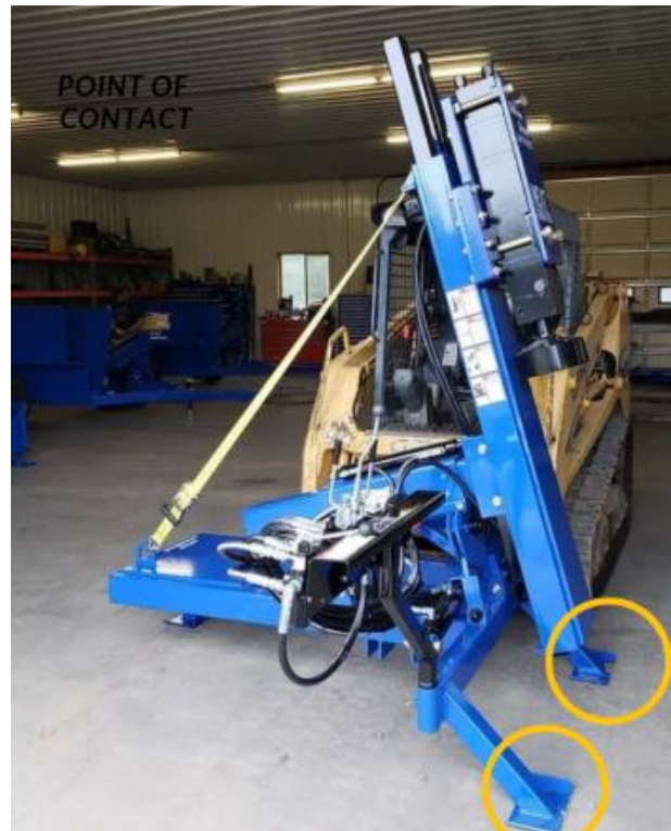
Photo 2. Photo showing type of skid steer mounted post-driver utilized in the incident. The yellow circles show the driver support arms. Photo obtained via Google image search.
