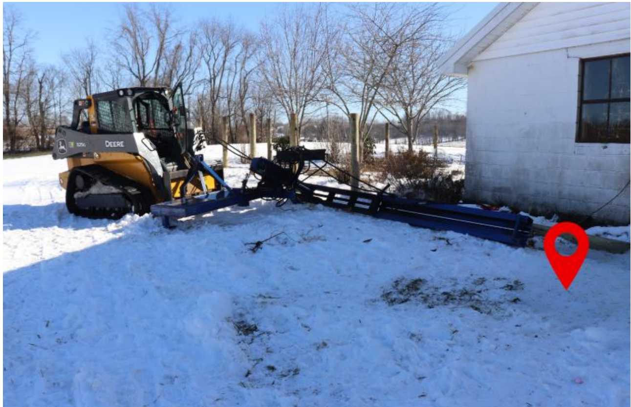
Photo 7. Photo showing failed post driver at the scene of the incident at final rest. Red location marker indicates location of the victim. Photo obtained via Kentucky open records request.
