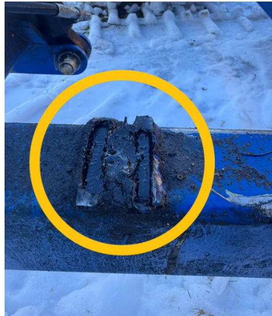
Photo 5. Photo showing post-driver attachment point and point of break. Photo provided by involved company.
